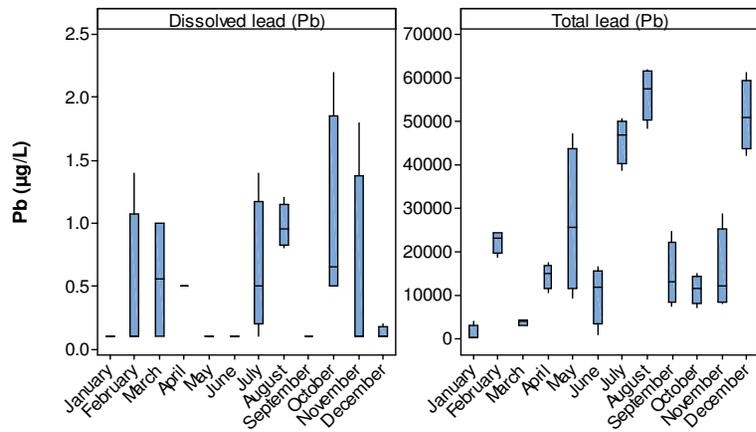
Figure 4-49 Monthly dissolved and total lead concentrations in tailings 2016 ( $\mu\text{g/L}$ )
