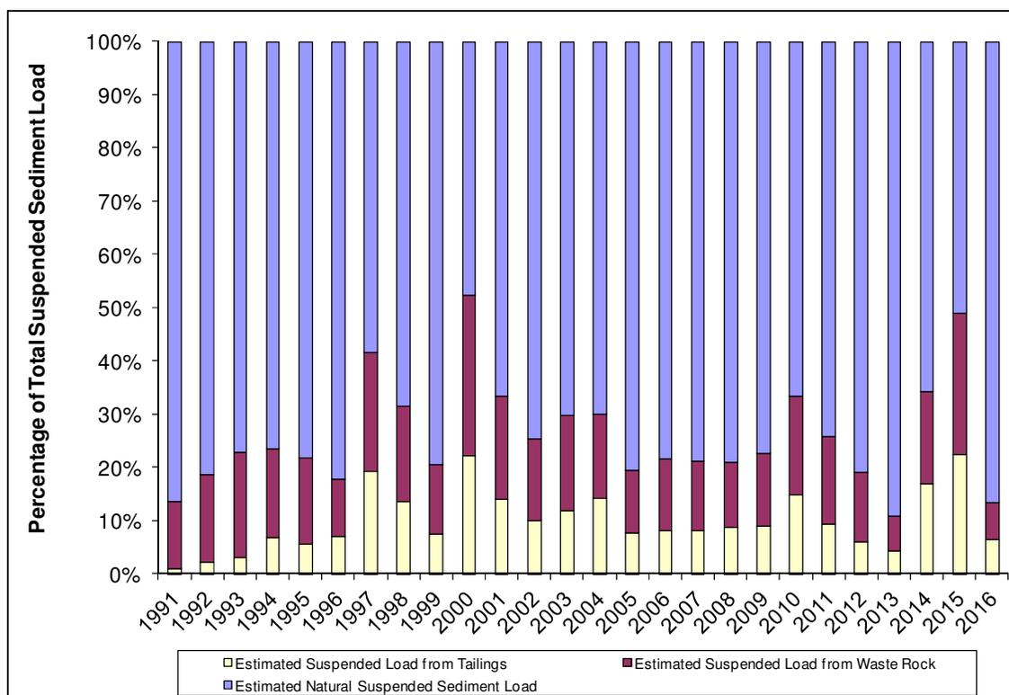
**Figure 7-8 Relative contribution of natural and mine-derived suspended sediment at SG3 (%) 1991-2016**
