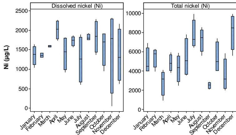
Figure 4-47 Monthly dissolved and total nickel concentrations in tailings 2016 ( $\mu\text{g/L}$ )
