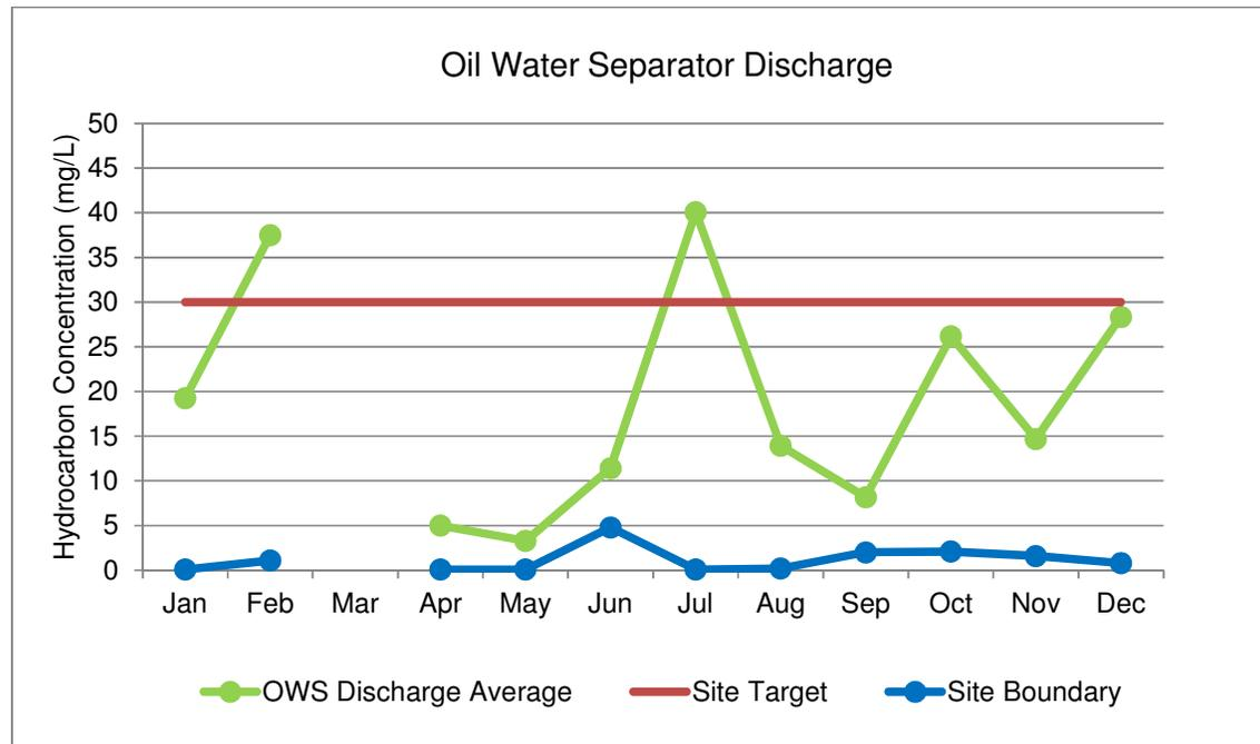
**Figure 4-60 Average monthly total hydrocarbon concentrations in oil water separator discharges 2016**
