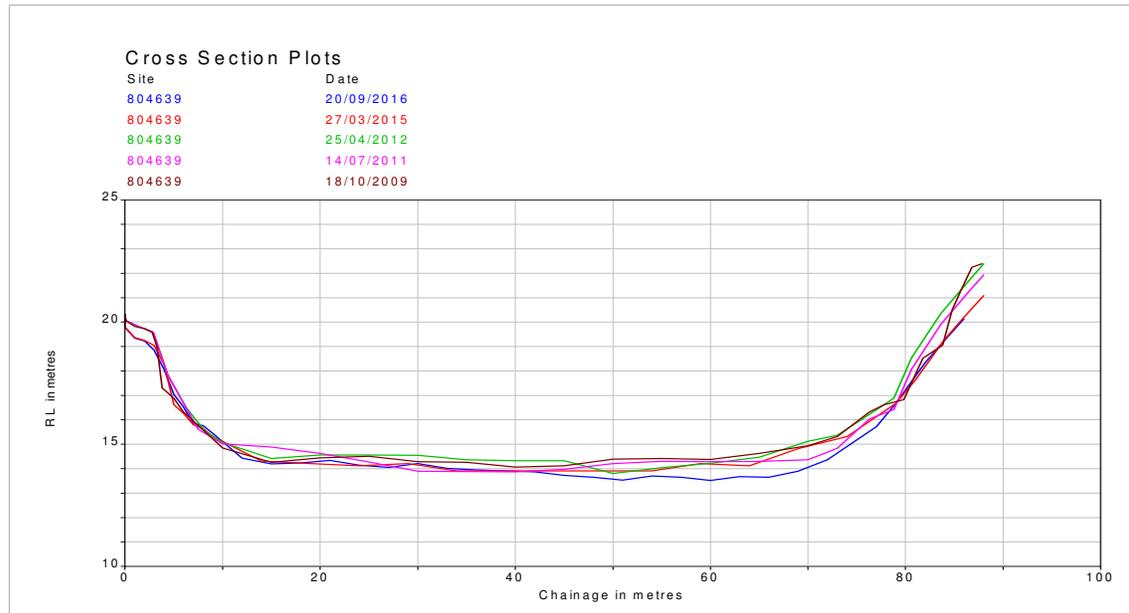
**Figure 7-13 Profile comparison (2009-2016) at Lagaip River at SG2**
