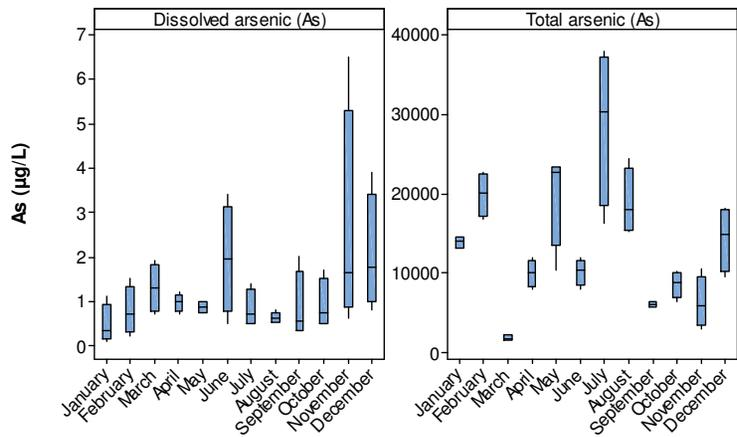
**Figure 4-35 Monthly dissolved and total arsenic concentrations in tailings 2016 ( $\mu\text{g/L}$ )**
