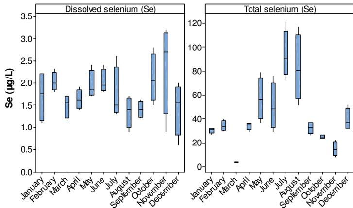
Figure 4-51 Monthly dissolved and total selenium concentration in tailings 2016 ( $\mu\text{g/L}$ )
