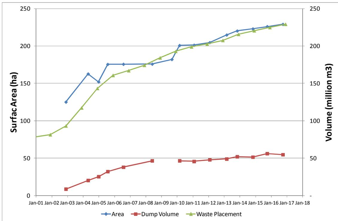
**Figure 4-13 Area and volume of Anawe Erodible Dump based on LiDAR survey 2001-2016**
