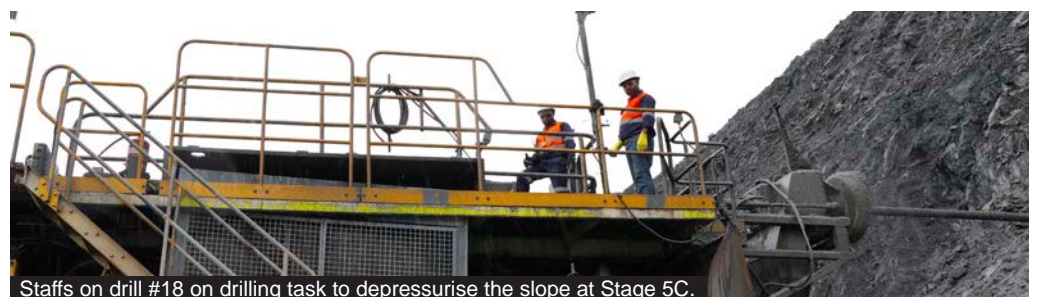
Staffs on drill #18 on drilling task to depressurise the slope at Stage 5C.
