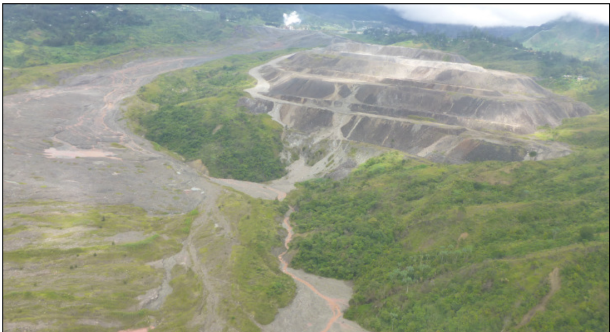
Figure 4-18 Anawe looking upstream showing runout from Anawe North Stable Dump
