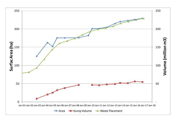
Figure 4-13 Area and volume of Anawe Erodible Dump based on LiDAR survey 2001-2016
