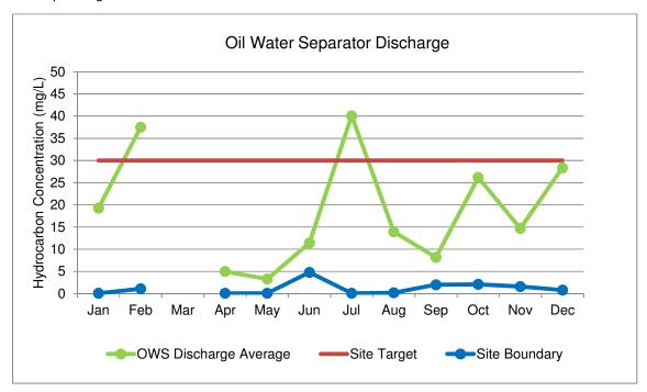
Figure 4-60 Average monthly total hydrocarbon concentrations in oil water separator discharges 2016
