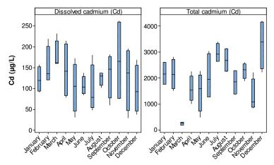
Figure 4-37 Monthly dissolved and total cadmium concentrations in tailings 2016 ( $\mu g/L$ )
