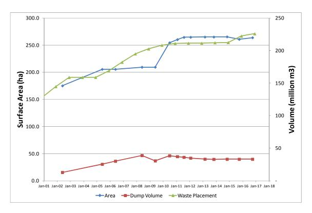
Figure 4-16 Area and volume of Anjolek Erodible Dump based on LiDAR survey 2001-2016
