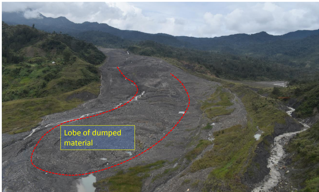
Figure 4-20 Dumped material 'rafting' downslope
