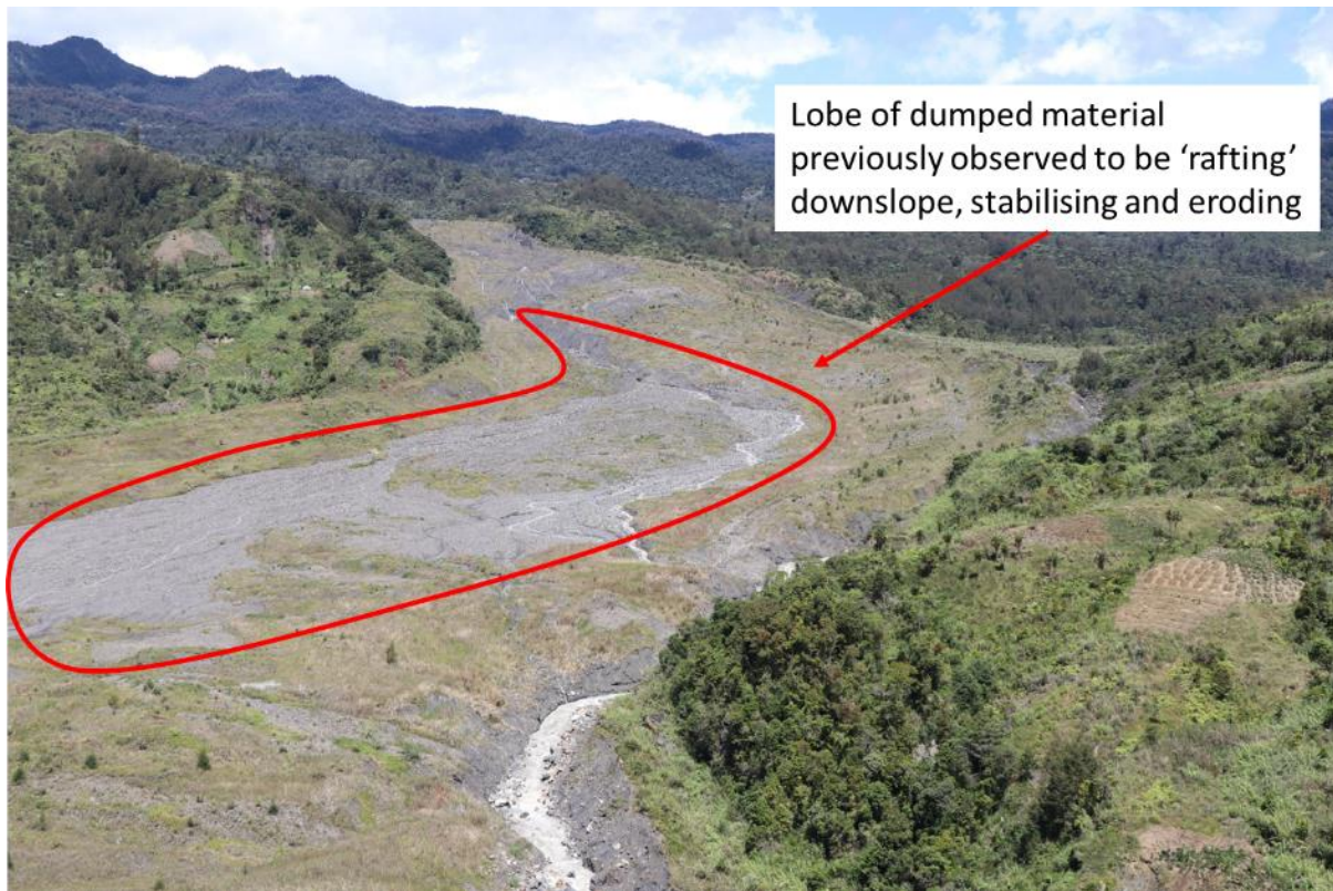
Figure 4-14 Anjolek erodible dump – lobe of previously dumped material stabilising and eroding – looking upstream August 2022
